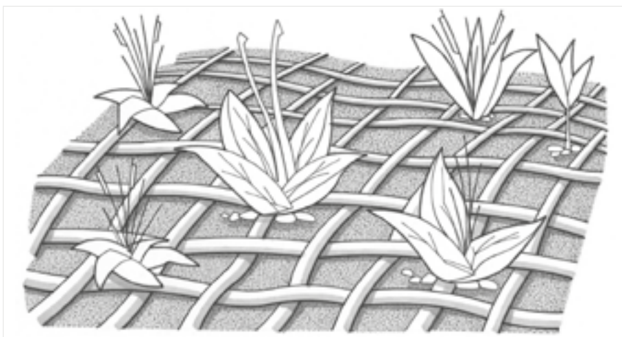
Figure 8: structure of a biotextile used for protecting a slope against erosion.
